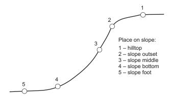
**Fig. 3.** Diagram for determining the situation of measuring points on a slope
