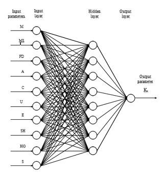
Fig. 4. Diagram of the MLP 10-8-1 model
